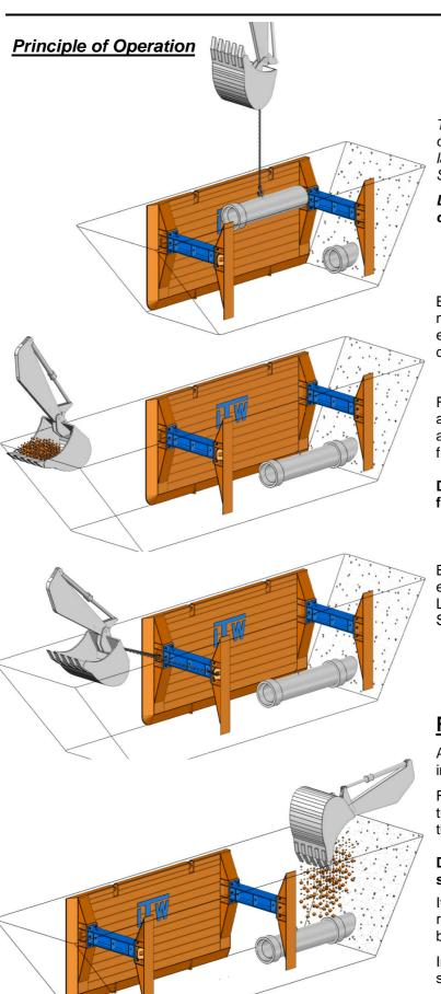
The Drag Box act as shield in the event of trench wall instability. Only the Pipe laying will be effected in between the Shield.
