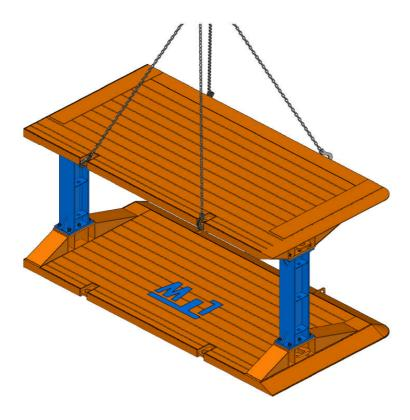
Use the lifting/transportation points at the top and the cutting edge to lift the second plate above the first plate. Tighten the screws as described above.
