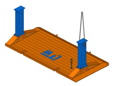
Place the Plate on the attachment points facing with the flange assembly upwards.
