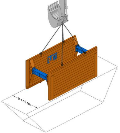
The pre-dug trench should be ~10cm wider than required trench width. The face sides are unprotected and need to be sloped depending on soil conditions.
